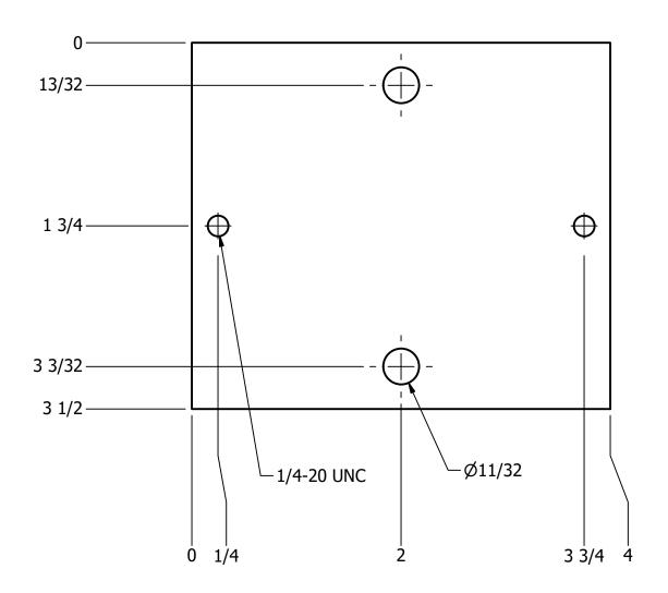
Panel Mount Plate\_EMT, top and bottom Make 18 1/8" Thick Galvanized or Cold Zink paint
